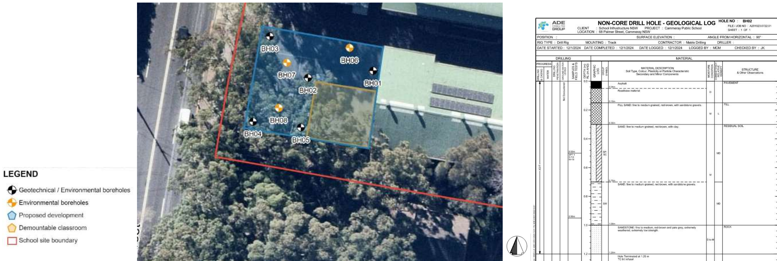
Figure 4: Borehole Locations & BH02 Log for Cammeray PS
